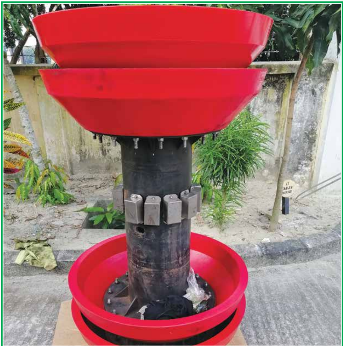
New pig before Pigging operation of Bakhrabad-Siddirgonj Gas Transmission Pipeline
